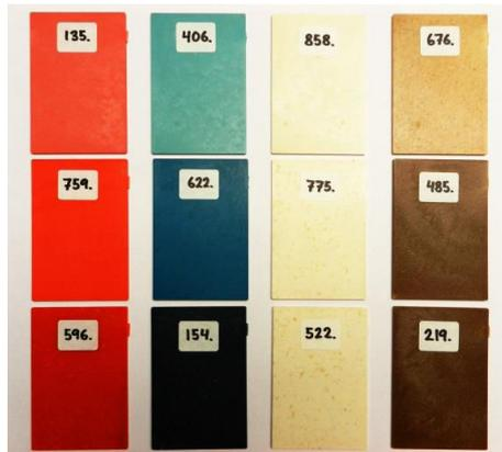
Figure 1 Example of wood fibre-reinforced polypropylene or polylactide composites used in the project.
