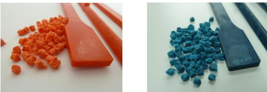
Figure 1: Coloured granules and test specimen
