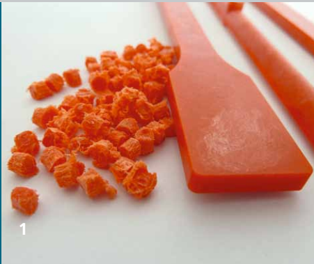
1 Coloured MouldPulp granulate and injected test specimen.
